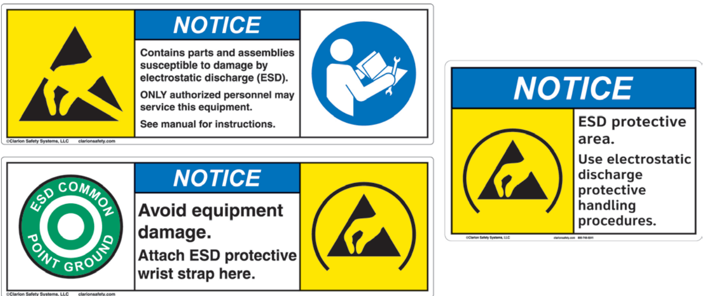
Figure 4: Examples of ANSI Z535-style ESD labels. (Designs ©2015 Clarion Safety Systems. All rights reserved.)
