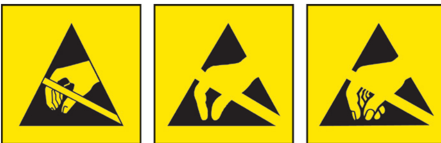
Figure 1: The ESD susceptibility symbol from ANSI/ESD S8.1 (at left), the simplified electrostatic sensitivity symbol from IEC 60417 (at middle) and the JESD471 symbol for electrostatic sensitive devices (at right).
