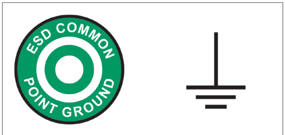
Figure 3: The common ground point symbol from ANSI S8.1 (at left) and the general earth (ground) terminal identification symbol from IEC 60417 (at right).
