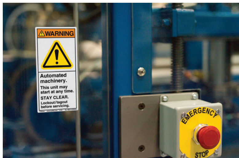
Figure 1: A typical emergency stop button on a machine (Label design at left ©2015 Clarion Safety Systems. All rights reserved.)
