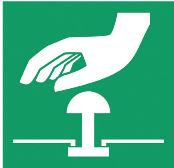
Figure 3: New ISO safety sign (symbol) for emergency stop
