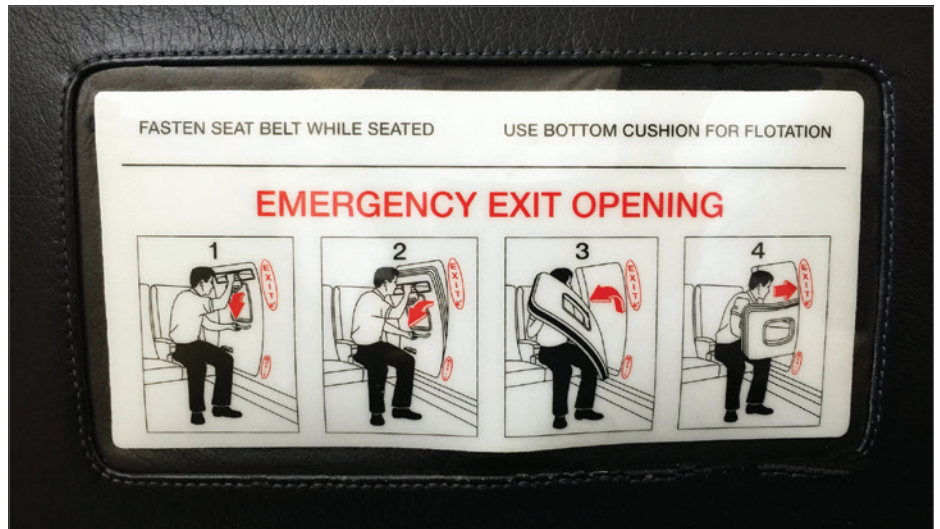
Figure 3: Example of step-by-step graphical instructions for an emergency situation on an airplane.
