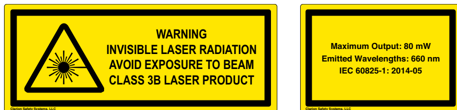
Figure 2A: Example of the still permissible older-style IEC laser safety label with separate explanatory information label
