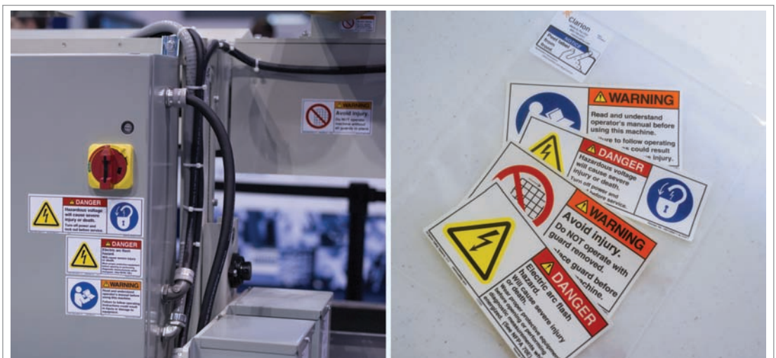
At left, multiple on-product safety labels reinforce each other, working as a "system" to convey essential safety messages. At right, a typical kit of safety labels. (Label designs ©Clarion Safety Systems.)
