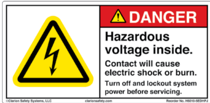
Figure 2: A typical ANSI Z535-formatted safety sign using the ISO electrical hazard symbol.
