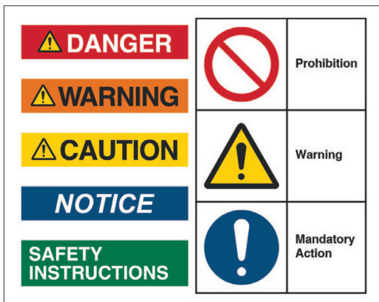
At left, signal word panels and their color-coding, per ANSI Z535.4. At right, examples of color-coding for the three types of symbols used in product safety labels.
